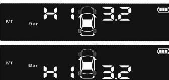
**Default setting:** Long press "M" menu key for 3 seconds until "U/S" (Unit setup) is displayed then short press "M" menu key several times to enter DE (Default setup) interface. Long press left/right keys for 2 seconds to restore default. Default reset is confirmed when "DF" appears on display.
