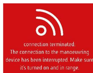
The connection to the App Controller was interrupted. Make sure the power is turned on. Reduce the distance to the Bluetooth module. If necessary, change the position of the module to improve reception. Open any aluminium-coated window blinds.
